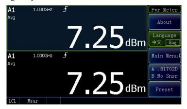
When the peak power sensor is connected, it is a high performance peak power meter. It can measure and analyze amplitude and time domain parameters of pulse modulated signals in the frequency range from 50MHz to 67GHz.
